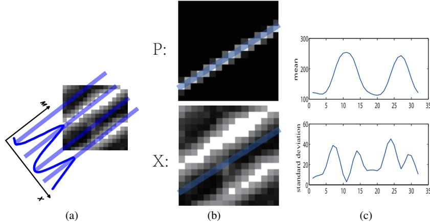
**Fig. 1** (a) Four sampling lines and sampled mean value. (b) The method of overlapping area to generate a sampling line: pixels' intensity is defined by the overlapping area between pixels and the sampling line.  $E[X]$  and  $Std[X]$  can be calculated by simply multiplying the matrix  $P$ ,  $X$  and  $X^2$ . (c) The sampled mean value and standard deviation from (b).
